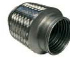
UFILOK57BMM Stainless steel flex-connector. Main body, stainless steel. End caps, aluminised steel L=101.6 mm/4". Fits over a 57 mm pipe.
