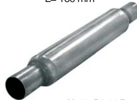
U 40 51 00R Silencer "MICRO 51" Round 76 mm, L=400 mm (excl. ends)
