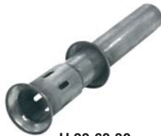
U 93 63 30 Decibel insert Should be placed inside piping in order to obtain an effective sound damping (note that this also leads to higher backpressure), L=275 mm
