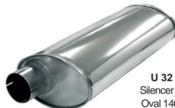
U 30 76 00R Silencer "TURBOTIGHT" Oval 140/220 mm L=250 mm (excl. ends)
