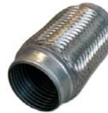
UFILOK635MM Stainless steel flex-connector. Main body, stainless steel. End caps, aluminised steel L=152.4 mm/6". Fits over a 2.5" pipe.
