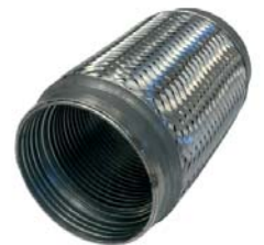
UFILOK1016203MM Stainless steel flex-connector. Main body, stainless steel. End caps, stainless steel L=203 mm/8". Fits over a 4" pipe.
