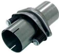
U 05 76 00 Compensator Should be used to prevent pipe fracture between the manifold and exhaust system, L=190 mm Stainless-Chromium steel
