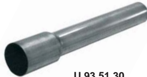
U 93 51 30 Decibel insert Should be placed inside piping in order to obtain an effective sound damping (note that this also leads to higher backpressure), L=283 mm
