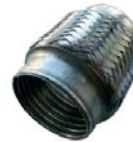
UFILOK635BMM Stainless steel flex-connector. Main body, stainless steel. End caps, aluminised steel L=101.6 mm/4". Fits over a 2.5" pipe.
