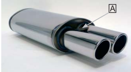
U 11 DJ DD Silencer "JETEX" Inlet pipe: 63.5 mm Oval silencer 140/220, L=420 mm Tailpipes Twin Round 80 mm, L=190 mm (excl. ends) Tailpipe width 165 mm Hanger point (A) 160 mm from end of taipipes
