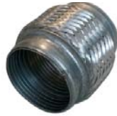
UFILOK765BMM Stainless steel flex-connector. Main body, stainless steel. End caps, stainless steel L=101.6 mm/4". Fits over a 2.5" pipe.
