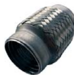
UFILOK48BMM Stainless steel flex-connector. Main body, stainless steel. End caps, aluminised steel L=101.6 mm/4". Fits over a 48mm pipe.
