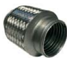
UFILOK45BMM Stainless steel flex-connector. Main body, stainless steel. End caps, aluminised steel L=101.6 mm/4". Fits over a 1.75" pipe.
