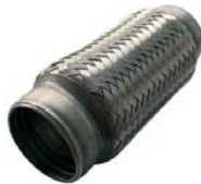
UFILOK48MM Stainless steel flex-connector. Main body, stainless steel. End caps, aluminised steel L=152.4mm/6". Fits over a 48mm pipe.
