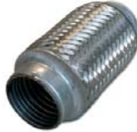
UFILOK515MM Stainless steel flex-connector. Main body, stainless steel. End caps, aluminised steel L=152.4 mm/6". Fits over a 2" pipe.
