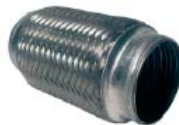
UFILOK45MM Stainless steel flex-connector. Main body, stainless steel. End caps, aluminised steel L=152.4 mm. Fits over a 1.75" pipe.
