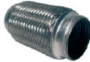
UFILOK765BMM Stainless steel flex-connector. Main body, stainless steel. End caps, stainless steel L=101.6 mm/6". Fits over a 2.5" pipe.
