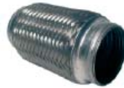
UFILOK635MM Stainless steel flex-connector. Main body, stainless steel. End caps, aluminised steel L=152.4 mm. Fits over a 2.5" pipe.
