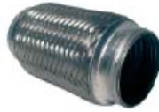
UFILOK765MM Stainless steel flex-connector. Main body, stainless steel. End caps, aluminised steel L=152.4 mm/6". Fits over a 2.5" pipe.
