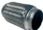
UFILOK515MM Stainless steel flex-connector. Main body, stainless steel. End caps, aluminised steel L=152.4 mm. Fits over a 2" pipe.
